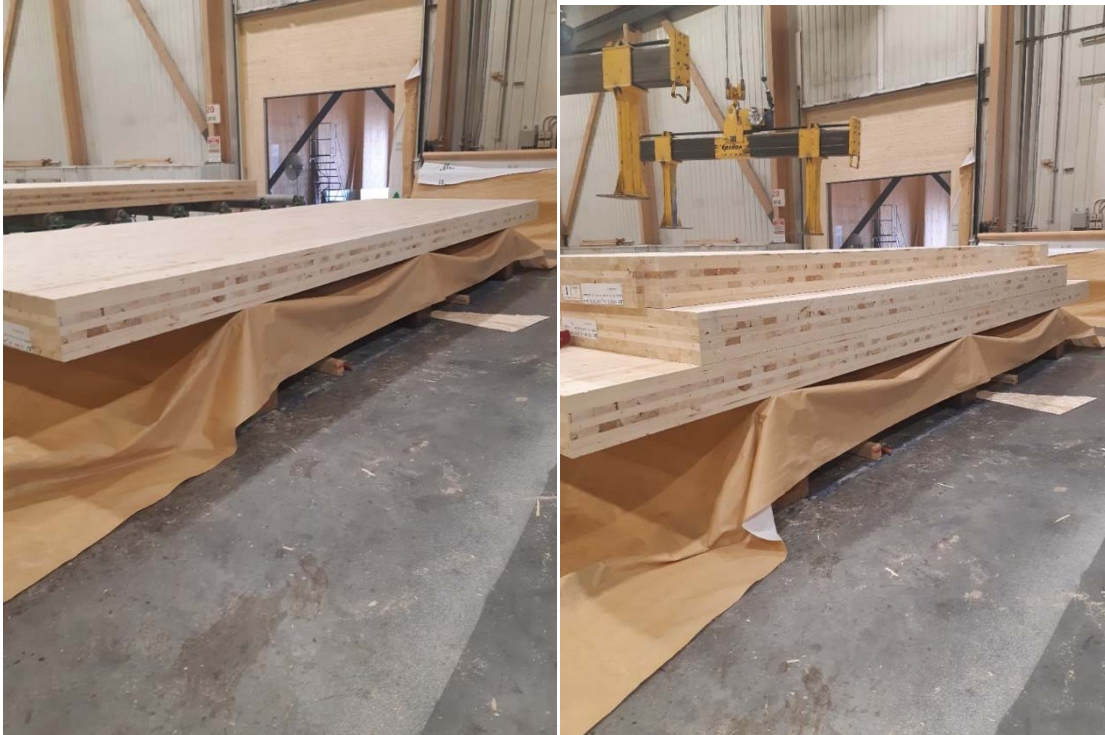
Figure 4.4 CLT panels are then stacked onto the wrapping, architectural face down. Oriented strand board (OSB) is inserted between the wrapping and the underside of the bottom panel to protect the OSB from damage in case of long-term storage.
