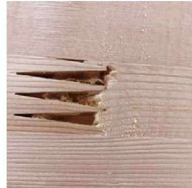
Figure 3.21 Hole in finger joint
