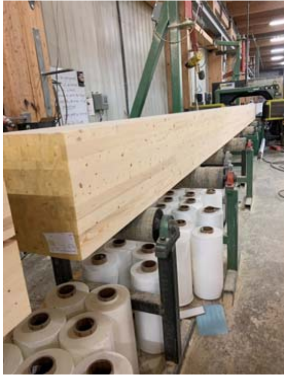
Figure 4.12 Glulam members are laid onto rollers.
