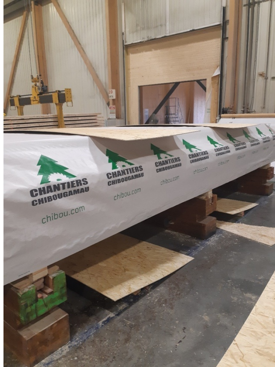
Figure 4.6 Oriented strand board (OSB) is then attached to the bottom of the package to provide protection when using a forklift.
