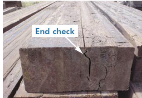
Figure 3.146 Types de gerces, extrait de l'APA EWS Technical Note: Evaluation of Check Sizes in Glued Laminated Timber, Form R475
