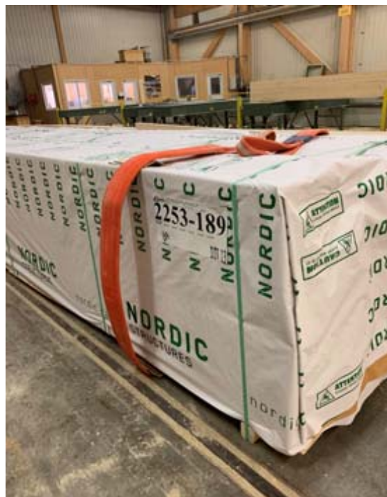
Figure 4.15 The entire package, including the lumber blocking that keeps the glulam elevated, is then strapped together. The packages are labeled, lifted, and stacked for storage.
