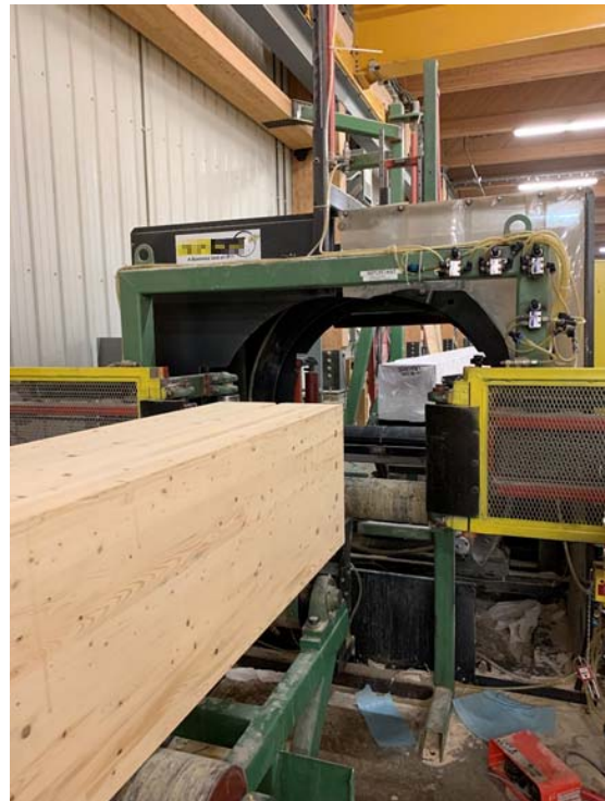
Figure 4.13 The rollers pass the member through a machine that wraps them up. After wrapping, cardboard angles are used to protect the corners of the members.
