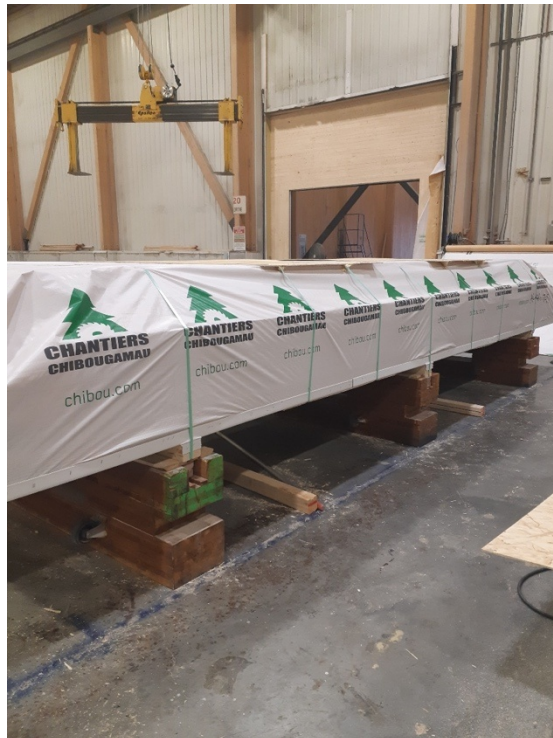
Figure 4.7 The entire package, including the lumber blocking that keeps the CLT elevated, is then strapped together.
