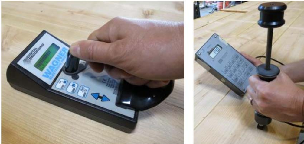
Figure 3.3 Measuring wood moisture content using a capacitance-based meter (left) and a resistance-based meter (right) (Source: FPI)
