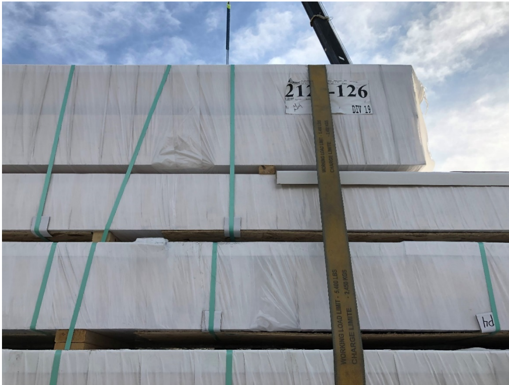
Figure 4.16 At the plant, cranes or forklifts are used to load the packages onto trucks; forklifts are used to load the packages onto trains. All packages are strapped down to prevent them from shifting during transport.
