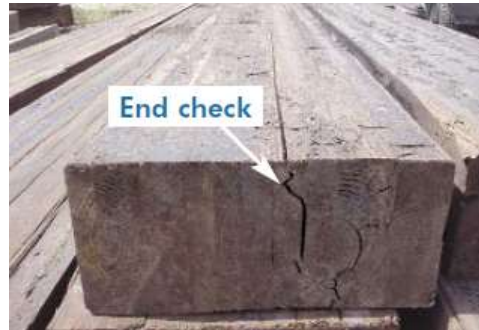
Figure 4.12 Types de gerces, extrait du document APA EWS Technical Note: Evaluation of Check Sizes in Glued Laminated Timber, Form R475
