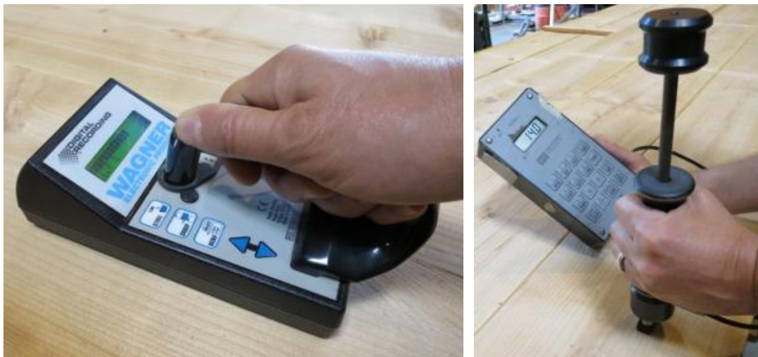
Figure 3.2 Measuring wood moisture content using a capacitance-based meter (left) and a resistance-based meter (right) (Source: FPI)
