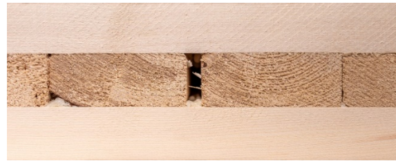
Figure 2.4 Gaps between adjacent lamination edges in an interior layer
