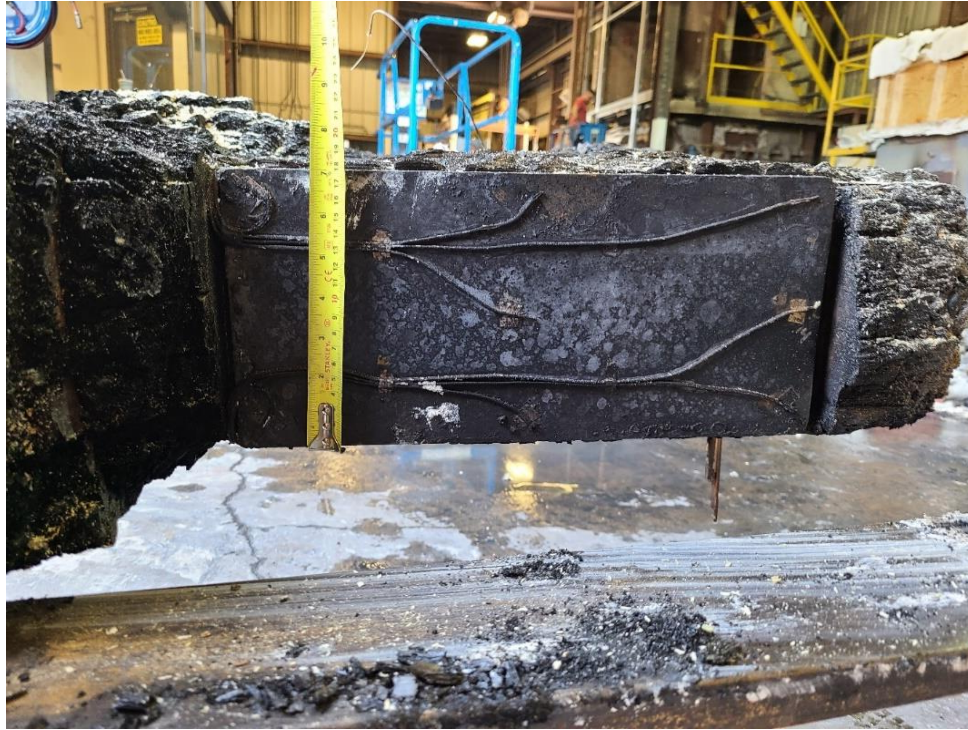
Figure 28: Bearing plate post-test
