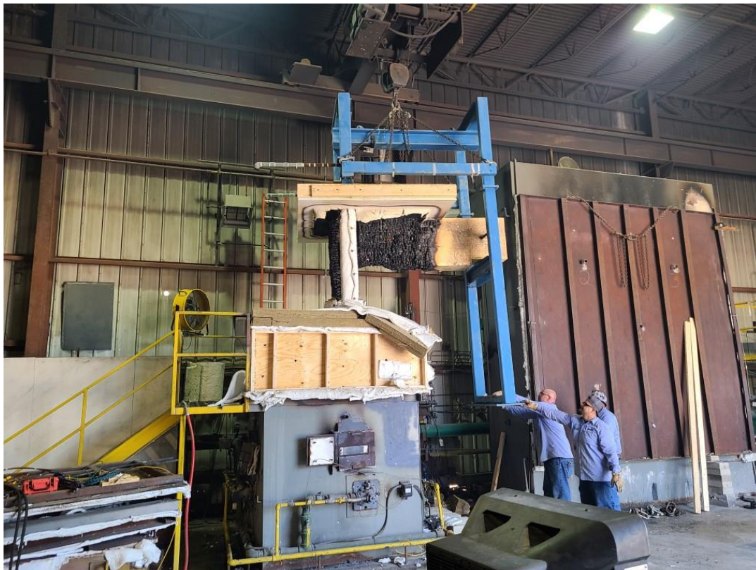
Figure 11: Test assembly being lifted out of furnace
