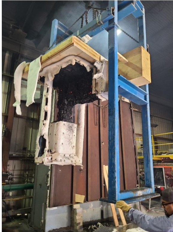
Figure 26: Test assembly being lifted out of furnace
