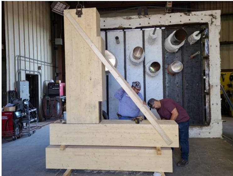
Figure 22: Beam (vertical) and column (horizontal) before hoisting
