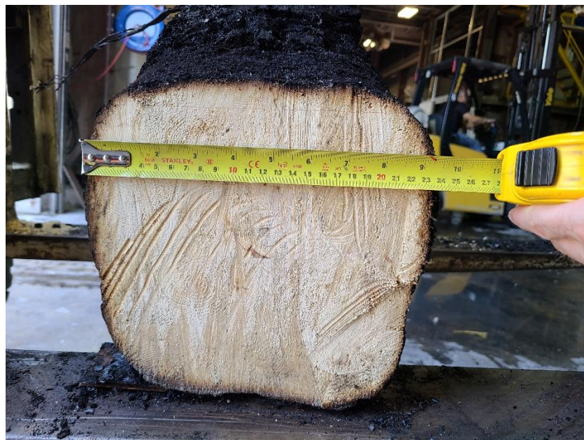
Figure 31: Column remaining cross-section post-test
