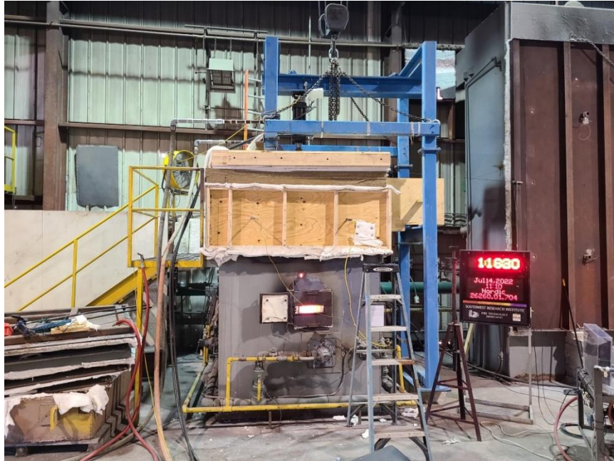
Figure 10: Furnace during testing
