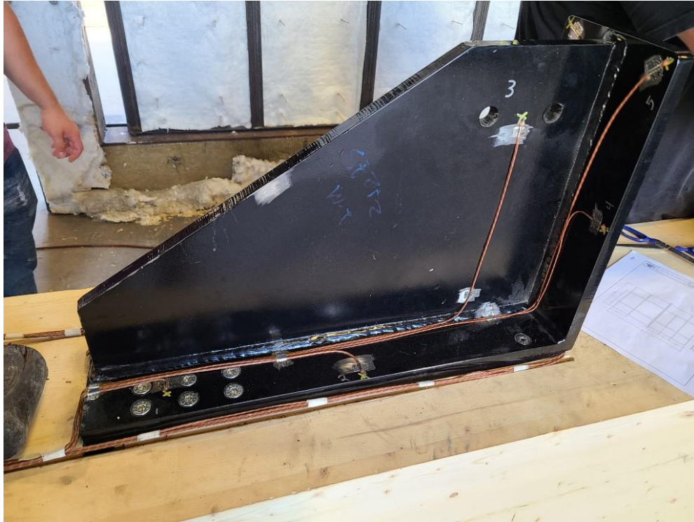
Figure 5: Bearing Plate with Thermocouples Installed
