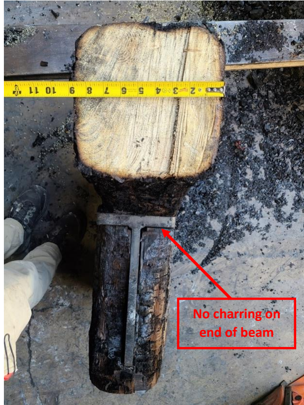
Figure 14: Column remaining cross-section post-test
