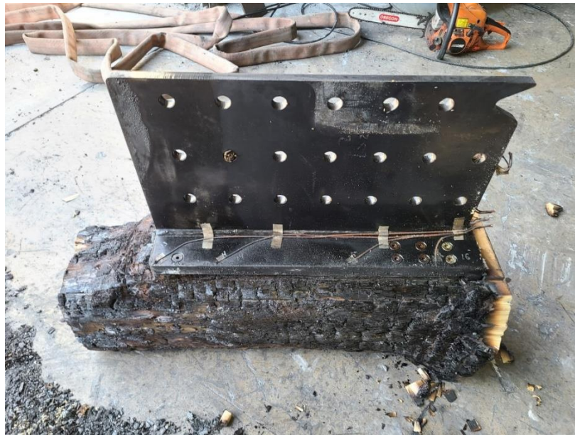
Figure 15: Knife plate-column connection post-test
