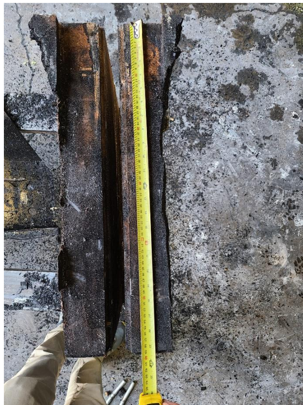
Figure 29: Beam remaining cross-section post-test
