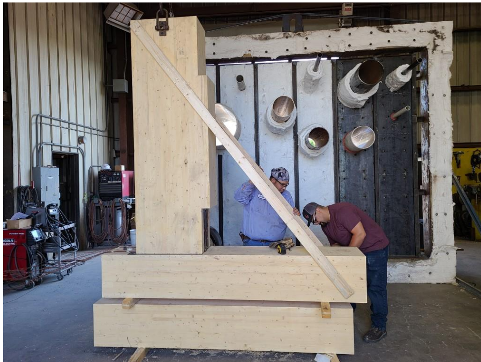
Figure 6: Beam (vertical) and column (horizontal) prior to installation of wood blocking
