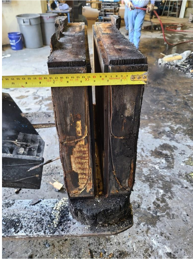
Figure 30: Bottom of beam post-test
