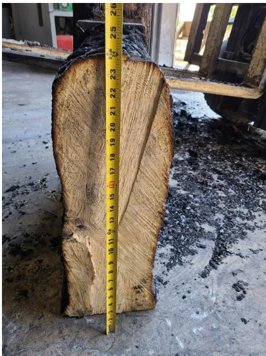
Figure 13: Beam remaining cross-section post-test
