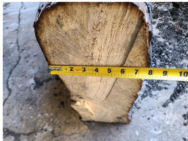
Figure 13: Beam remaining cross-section post-test
