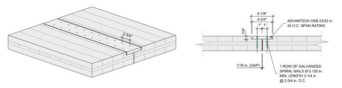
ASD Allowable Shear Capacity: 1,000 lbf/ft | LRFD Factored Shear Resistance: 1,400 lbf/ft
