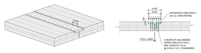
ASD Allowable Shear Capacity: 1,500 lbf/ft | LRFD Factored Shear Resistance: 2,100 lbf/ft
