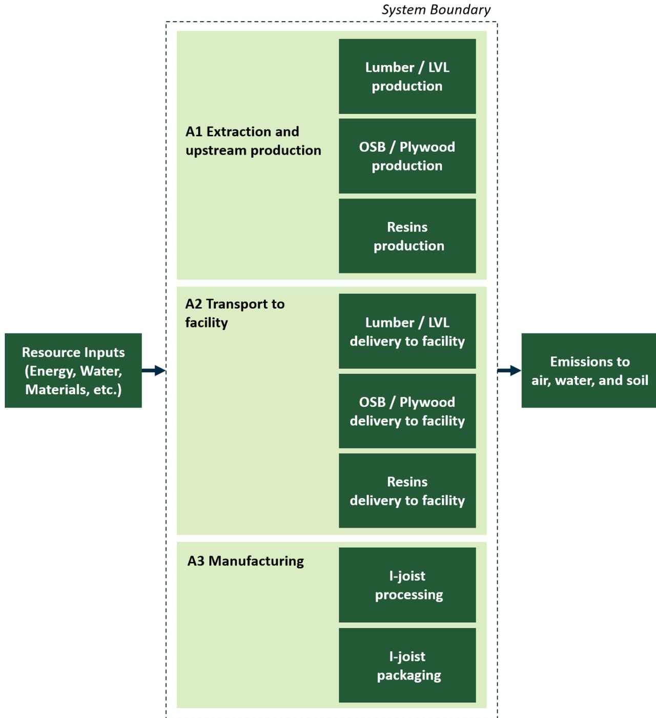
Figure 1. Cradle-to-gate I-joist production flow diagram
