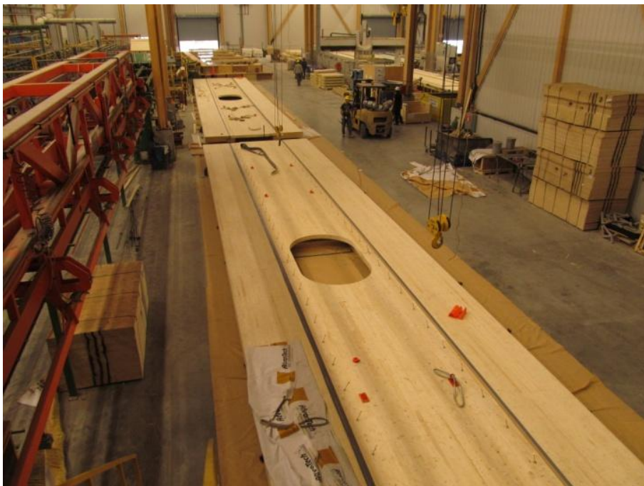
Figure 15: Fabrication of a principal beam
