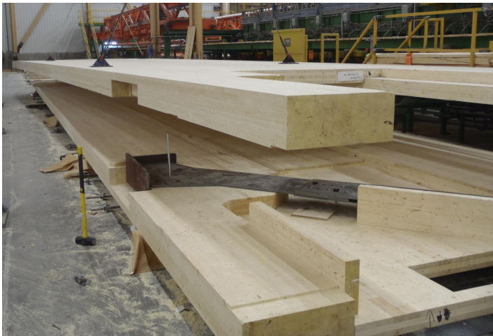
Figure 17: Fabrication of a principal beam, gluing half-parts together
